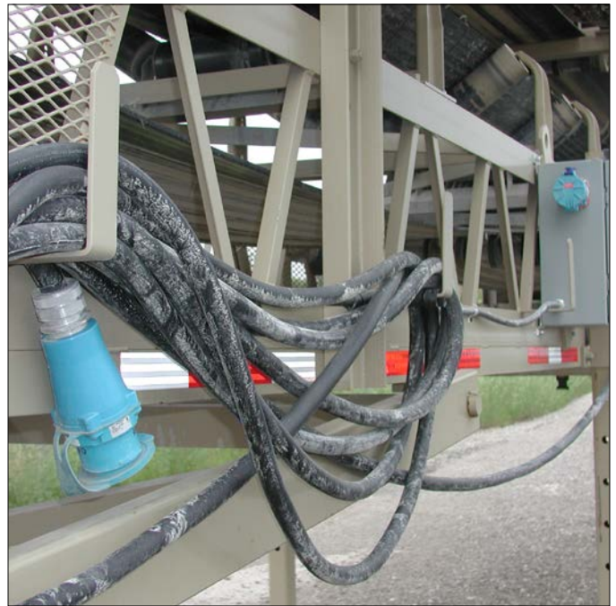
A typical portable conveyor setup includes a MELTRIC plug and connector on panel and power cord. MELTRIC's easy twist connection is not affected by grit like the threaded nut on previous pin-and-sleeve connectors.
