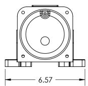
TOLERANCES UNLESS OTHERWISE SPECIFIED **ENGLISH** DRAWING TITLE: DX30 METAL WALL BOX 0.X ±0.05 0.XX ±0.01 SCALE NTS DATE: MATERIAL: **METAL** REMOVE BURRS & SHARP EDGES TO .015 MAX. 0.XXX ±0.005 PROJECT NUMBER PART NUMBER SHEET: DIMENSIONS SHOWN IN OVALS ARE INSPECTION DIMENSIONS. NONE 26-3A023-xx 1 OF 1
