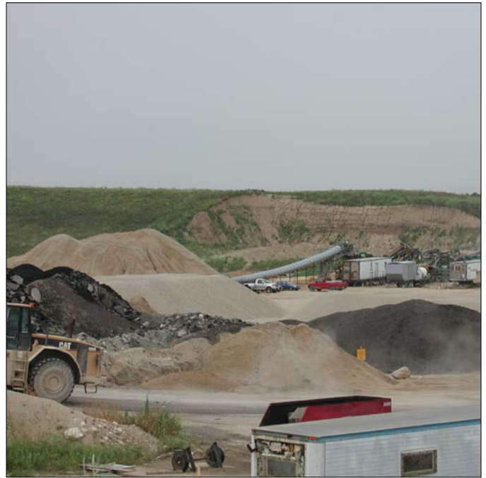
Portable conveyors and crushers at this Payne & Dolan aggregate operation are easier to move as they follow the material source because MELTRIC plugs and receptacles simplify power connections.
