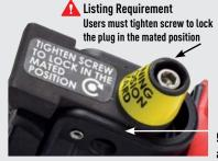
Zone 2/Division 2 DS100C receptacles feature a standard screw-type locking pawl. This required feature allows the user to lock the plug to the receptacle by tightening a screw on the pawl.
