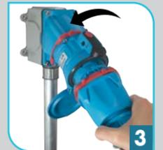
Rotating the de-energized plug 30° counterclockwise closes the safety shutter and frees the plug to be withdrawn from the receptacle.
