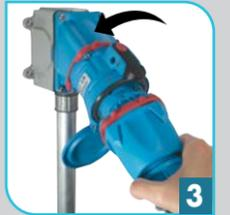
Rotating the de-energized plug 30° counterclockwise closes the safety shutter and frees the plug to be withdrawn from the receptacle.
