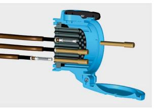
To insert contacts when they have been wired is simple. Push wired contact into rear of insulator until it stops to complete the installation.
