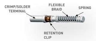
After terminating the contact, simply insert it by pushing the contact into the back side of the interior insulator until it reaches a positive stop. The contact may be inserted and removed up to three times for future rewiring.
