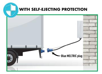
Hazards to personnel and equipment damage are eliminated when the truck or other mobile is equipped with a self-ejecting device, which will disconnect power and release connectors safely.
