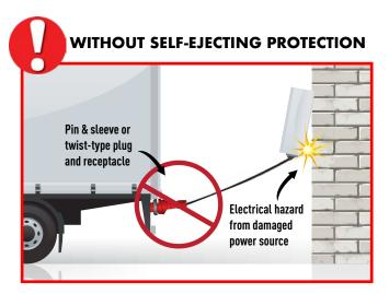
The potential of hazards to personnel and equipment damage are **created** when a truck or other mobile vehicle moves prior to manually disconnecting electrical power.
