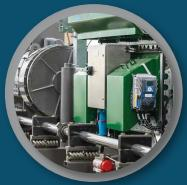
A MELTRIC DS200 is shown providing power to pumps found on an electronic fracking system, producing significantly lower emissions compared to the diesel driven pumps.
