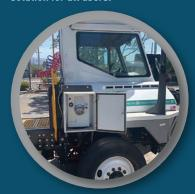
MELTRIC DS200 is a Switch-Rated 200 A device being used to recharge the EV battery on this industrial truck.
