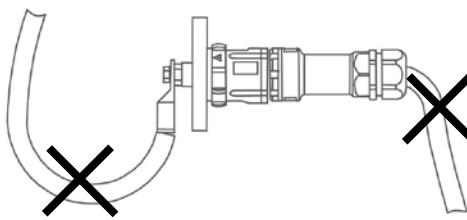
**NOTICE:** Ensure the plug and its flexible cable do not exert a significant force or a constraint on the receptacle.
