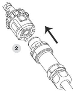
Pull on the plug to make sure it is properly latched in the receptacle. Figure 3 A small rotation of the plug, in either direction, engages the locking finger on the receptacle to prevent any further rotation.
