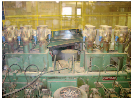
Closeup shows typical motors with Meltric Decontactors in place. Dead-front construction keeps workers safe, while plug-and-play simplicity speed motor removal and reinstallation.
