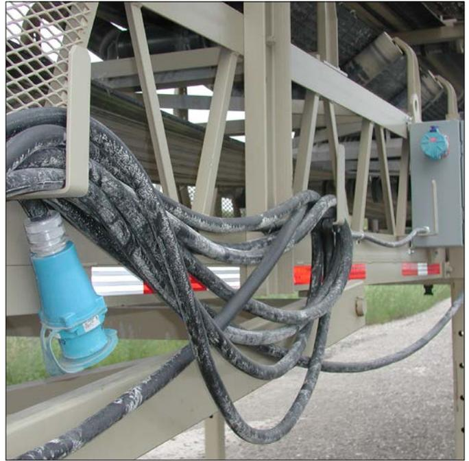
Typical portable conveyor setup includes MELTRIC plug and connector on panel and power cord. Easy twist connection is not affected by grit like the threaded nut on previous pin-and-sleeve connectors.
