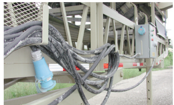
Typical portable conveyor setup includes Meltric plug and connector on panel and power cord. Easy twist connection is not affected by grit like the threaded nut on previous pin-and-sleeve connectors.
