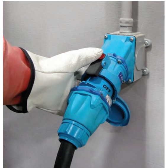
Meltric’s Decontactor plugs and receptacles are an NEC-approved ‘line of sight’ disconnect switch. Depressing the pawl on the receptacle (red dot) breaks the connection and ensures that the plug can be safely removed from the receptacle.
