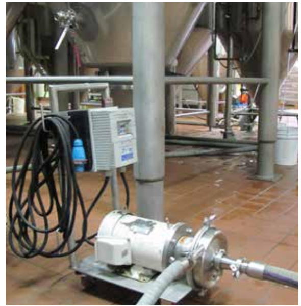
Founders Brewery uses Meltric Decontactor Series switch-rated plugs and receptacles on brewery production equipment such as mobile pump carts, keg washers, motors and other portable equipment. Any qualified worker can connect or disconnect a plug. Making and breaking connections with Decontactor plugs is a Risk Category '0' operation so the need for the cumbersome PPE when working near live parts is eliminated.
