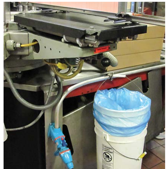
Meltric DECONTACTOR™ Series switch-rated plugs and receptacles can safely make or break electrical loads. They are a NEC-approved 'line of sight' disconnect switch, as shown here on a glass bottle labeling machine.
