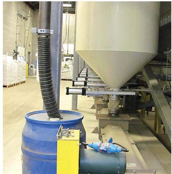
*Bell's Brewery has the benefit of limiting downtime on their grain handling equipment, associated with maintenance and motor change-outs, since no hardwiring of connections is necessary.*
