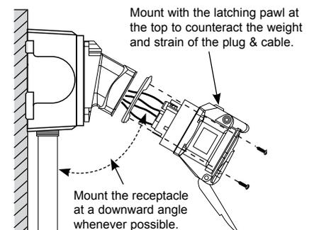
Insert the cable or wires through the wall box and cut to allow adequate length. Strip the cable sheath as
