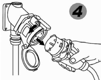
Rated ingress protection applies to the device when the plug and receptacle are mated and latched together. It also applies to the receptacle when the lid is latched closed.
