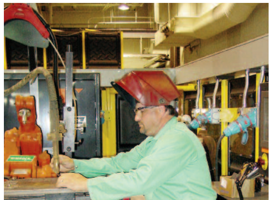
Welding technician Tim Moore prepares a GMAW torch on a mechanized fixture.
