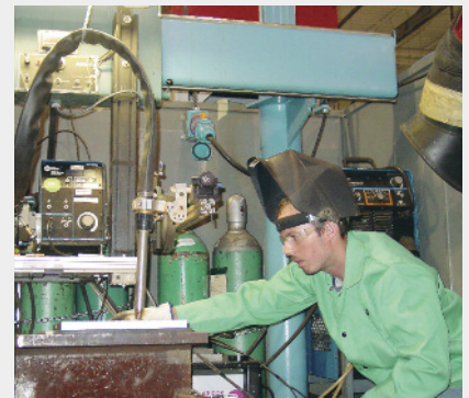
Switch rated plug and receptacle (background) enables technician to safely deenergize and relocate welding equipment.
