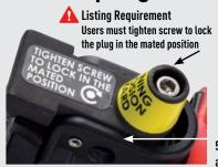
Zone 2/Division 2 DS20 receptacles feature a standard screw-type locking pawl. This required feature allows the user to lock the plug to the receptacle by tightening a screw on the pawl.
