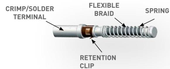
After terminating the contact, simply insert it by pushing the contact into the back side of the interior insulator until it reaches a positive stop. The contact may be inserted and removed up to three times for future rewiring.
