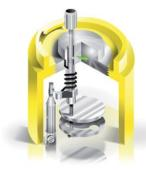
After depressing the pawl, the plug is rotated in a counterclockwise direction. This frees the switching contact for operation and the release of the remaining spring tension causes a quick breaking of the contacts. The plug may now be removed, if desired.
