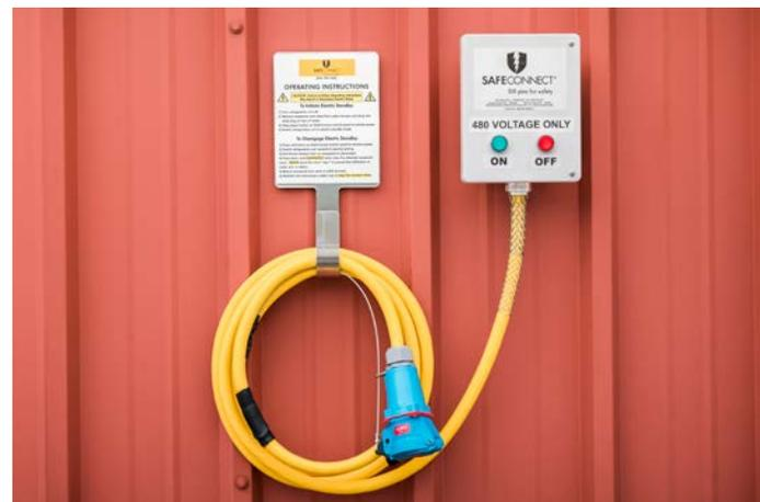
In the event of an operator error, such as a driver neglecting to press the "OFF" button before disconnecting, no harm will occur to the operator, the plug, or the receptacle. Any disconnection, even while under load, will completely de-energize the entire system before a dangerous electrical arc can develop.
