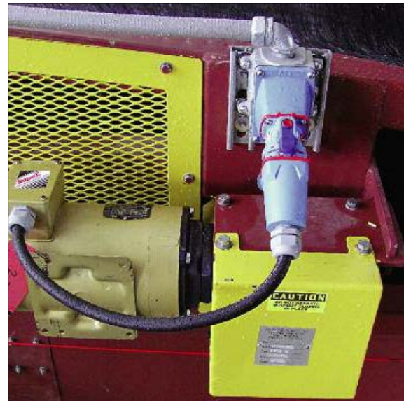
Installing a MELTRIC Switch-Rated plug and receptacle between a motor connection box and the power line feed eliminates all hardwiring tasks during motor changeouts. Load breaking is performed in seconds by pushing the pawl on the plug's casing.
