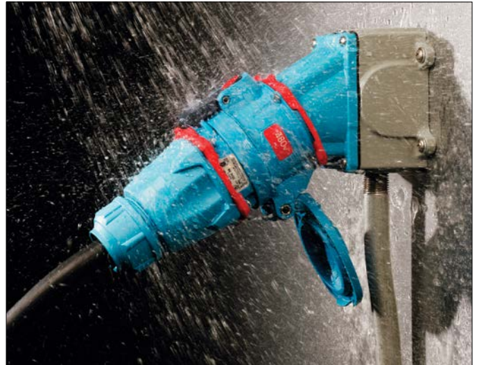
Washing down equipment is a frequent activity at ZD Wines. MELTRIC Switch-Rated plugs and receptacles are automatically Type 4X watertight whenever they are mated together.
