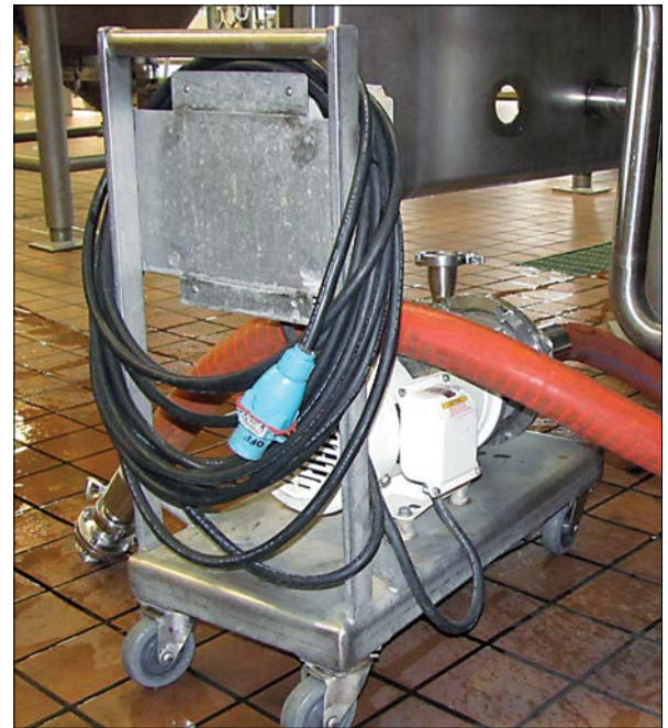
At Bell's Brewery, portable pump carts are connected with MELTRIC Switch-Rated plugs and receptacles. Silver-nickel contacts provide reliable corrosion-free connections, even in harsh conditions.
